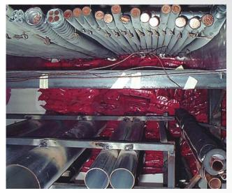
SpecSeal® Super System UL pre-test assembly
