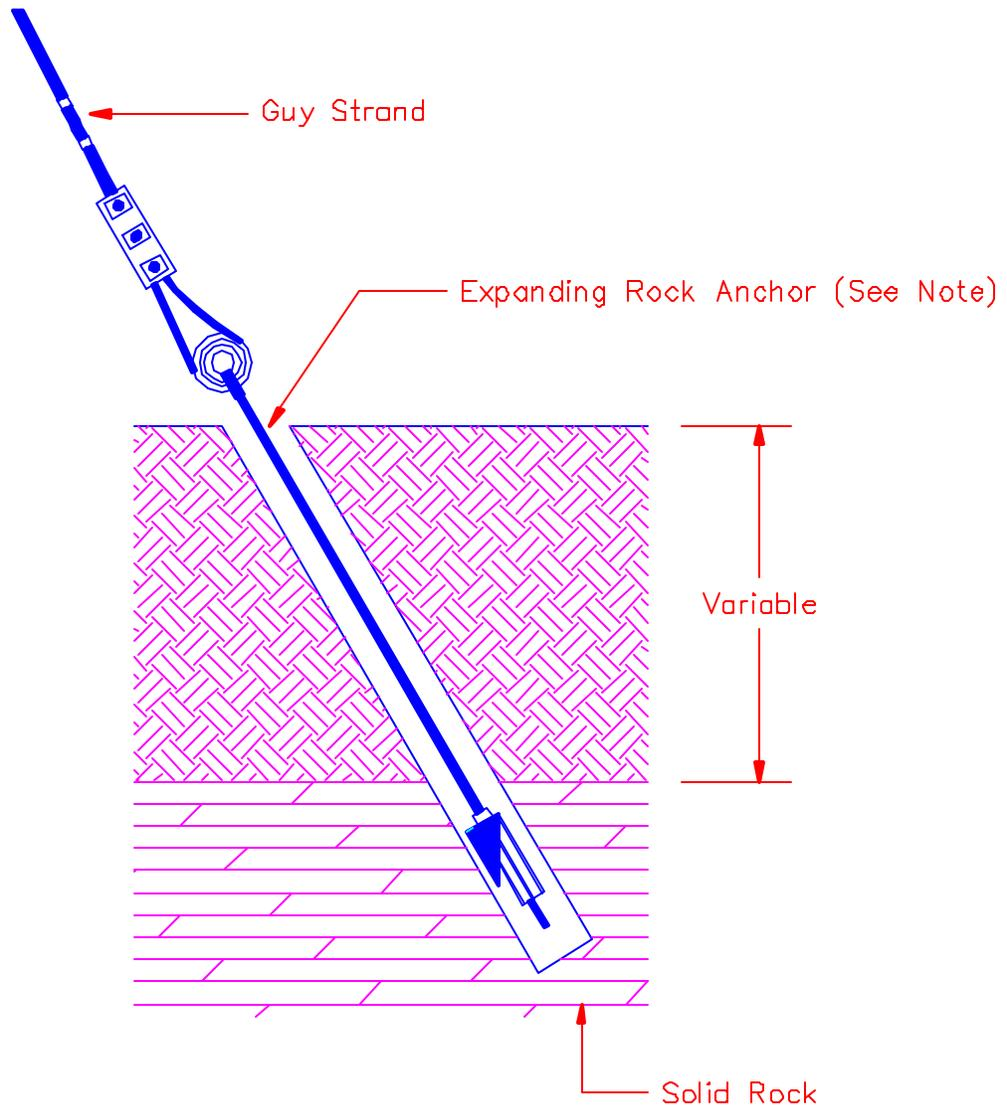
Note: The anchor should be installed in line with the guy strand.
