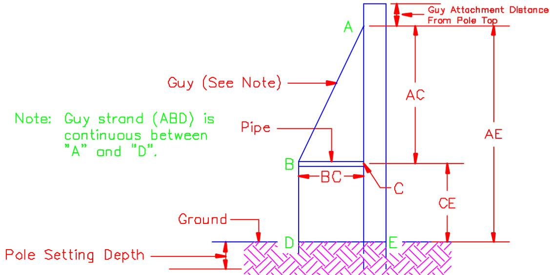
Procedure For Determining Guy Size And Pole Class For Sidewalk Guy
