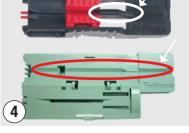
2.05 For 250µm: Mark 35mm from the end of the fiber. Strip the fiber to the mark. Clean the bare fiber. (see *Figure 5*)
