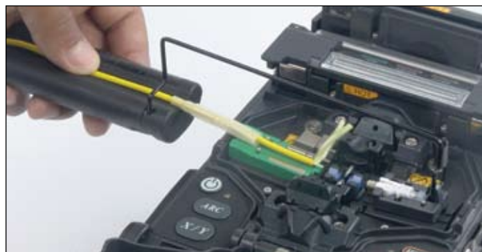
FIGURE 7 — Insert Transfer Tool into Connector Body Holder
