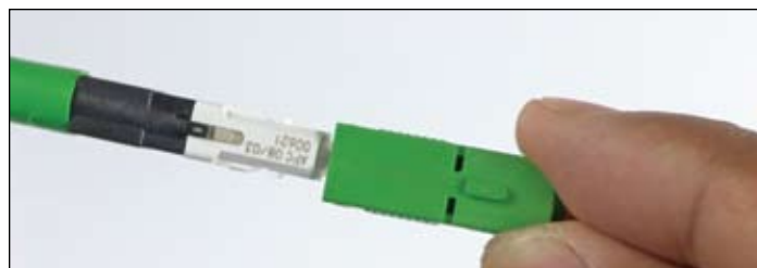
FIGURE 10 — Installing Connector Housing onto Connector
