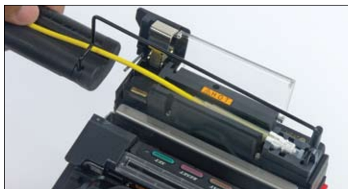
FIGURE 8 — Inserting Connector Body into Tube Heater
