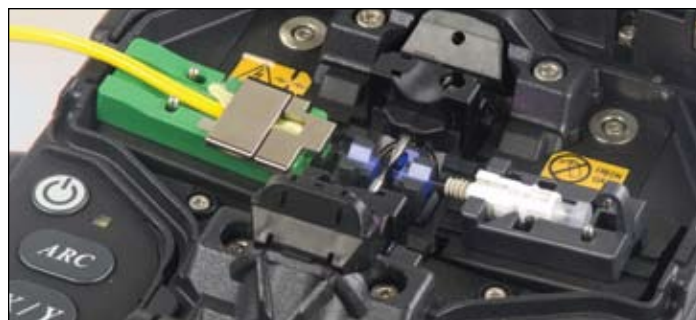
FIGURE 6 — Placing Fiber Holder & Connector into Splicer
