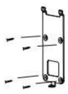
(4) Fix the back plate on the wall according to the mounting paper.
