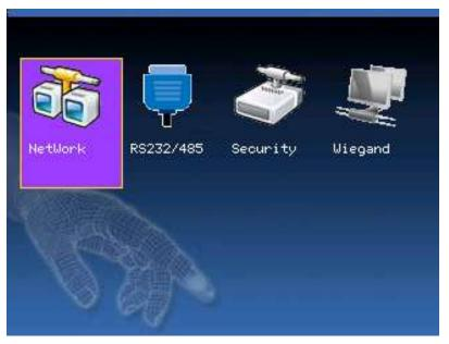
From within the Comm Menu, scroll with the  $\triangleleft / \triangleright$  keys until **Network** is highlighted. Press the **OK** key to accept.
