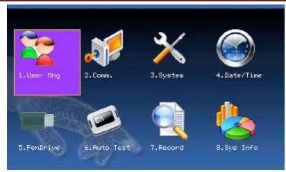
From the Main Menu, highlight and select **Comm.** to configure Communication Settings. Then press the **OK** Key to accept
