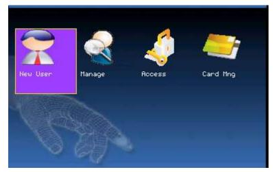
Scroll with the  $\blacktriangle/\checkmark$  keys and highlight **Manage**. Then press the **OK** key to open the User Manage screen:
