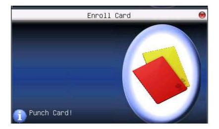
Flash the card near the keypad of F18 reader, press OK key to save after the device reads and displayes the card number.
