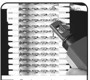
Terminate each conductor using an S814 impact tool or equivalent.
