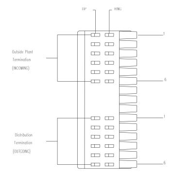
Terminal shall be installed to the applicable requirements of the: National Electrical Code, ANSI/NFPA 70(Article 800, Section C) Canadian Electrical Code, Part 1 (Section 60)
