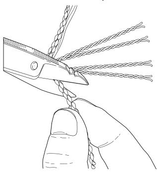
Twist ends back together for connecting hardware terminations
